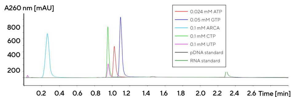
**Figure 1: Overlay of IVT mixture components on CIMac PrimaS** (product number 110.5118-2), Buffers: MPA (50 mM HEPES pH 7), MPB (50 mM HEPES, 200 mM sodium pyrophosphate, pH 8.5). Method: 0–1 min (100 % MPA), 1–1.8 min (gradient to 20 % MPB), 1.8–2.5 min (gradient to 80 % MPB). Full method not shown. PATfix™ HPLC system, UV absorbance at 280 nm, flow rate 2 mL/min, injection volume 25 µL.
