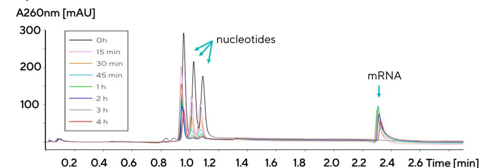
**Figure 3: Time-point analysis of nucleotide and mRNA content during IVT progression.** Sample: IVT sample, inactivated with EDTA and diluted in MPA (200-fold dilution).
