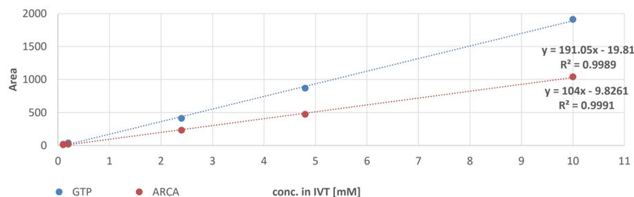
**Figure 2: Standard curves for ARCA and GTP peak areas.** Plot showing Area vs concentration of ARCA and GTP in IVT (200-times diluted; injected 25 µL). The method is linear in the selected range. Other calibration curves not shown here.
