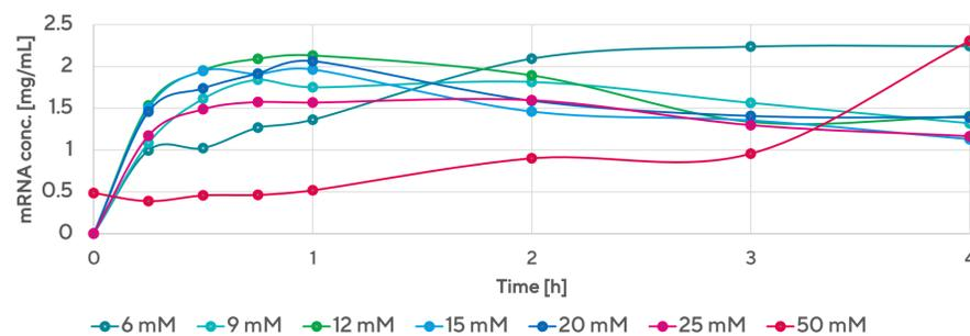
**Figure 4: Kinetics of the IVT reaction at different concentrations of MgCl<sub>2</sub>.** Samples: IVT sample, inactivated with EDTA and diluted in MPA (200-fold dilution).
